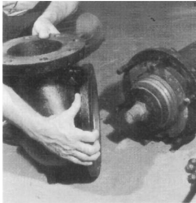
5. Position Shoe to slip in place.
