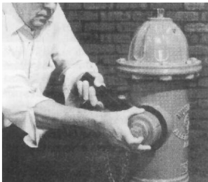
3. Place Nozzle Wrench, A-316, on Nozzle with Wrench Forks facing toward Hydrant Barrel and locked onto Nozzle Drive Lugs. Replace Nozzle Cap and tighten until Cap rests loosely against backside of Wrench.
